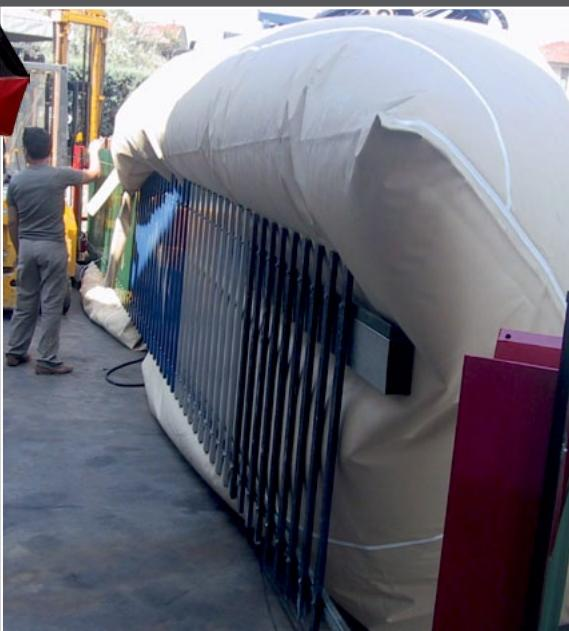
The vertical AVANTGATES are tested for resistance to wind load and CERTIFIED IN CLASS 4 (up to 152 Km/h), according to the European Regulation EN 12424. This makes the Avantgates able to be installed even in those areas where intense wind could be expected.
